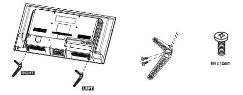
3. Insert the TV stand screws into the designated holes in the rear of the TV base stand and tighten the screws firmly with a Phillips Head screwdriver (not included).
